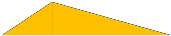
Figure 7: Cross section of the slopes: Steep southern slope is covered with Plastic sheet to prevent soil erosion; Topsoil below the plastic sheet is scrubbed and placed on the northern slope
